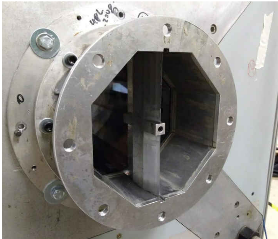
Figure 14: Wind tunnel extension and vertical support strut affixed to the aft-end of the MSBS.
