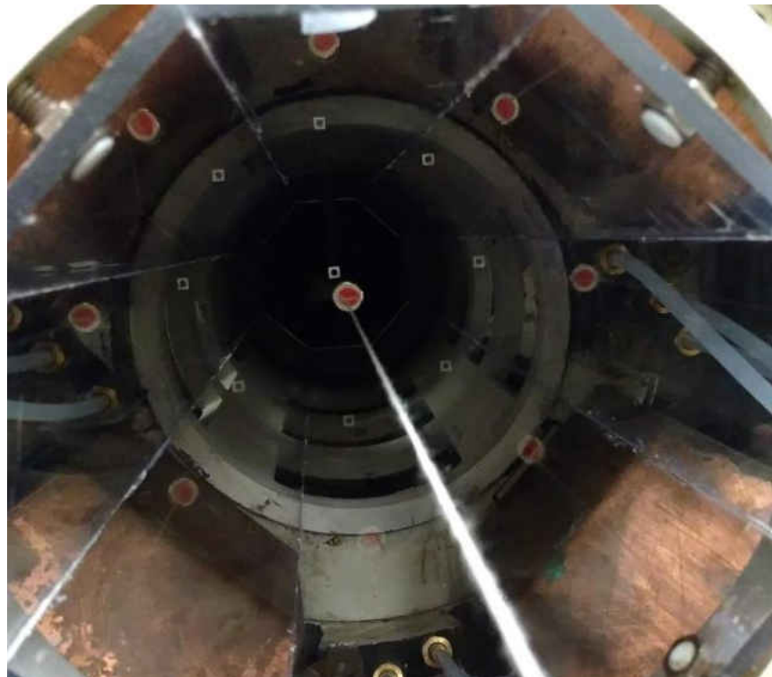
Figure 24: Permanent magnet core under applied load during drag loading test.
