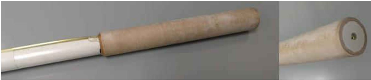
Figure 13: Second dummy sting with cavity pressure tap.
