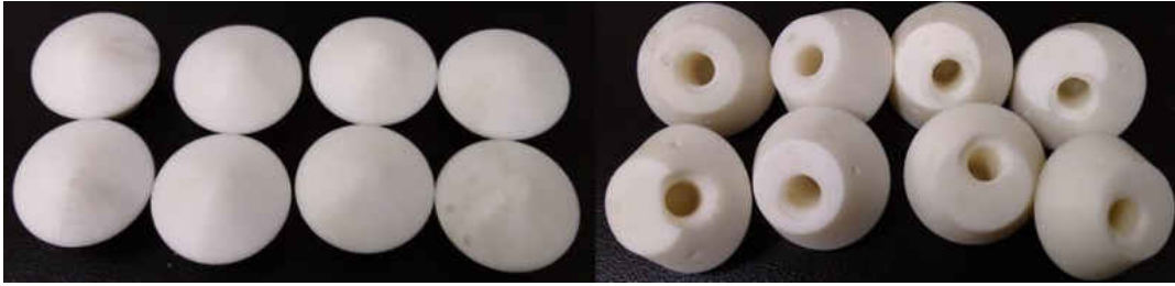
Figure 16: Fore and aft views of the sting supported models.
